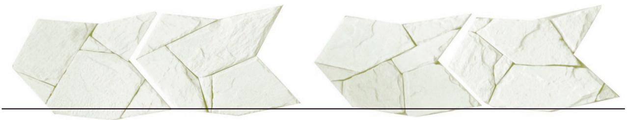
Cut along lowest point to begin installing with a flat base
